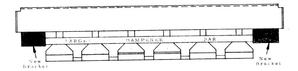
TO PREVENT THE STEEL BALL FROM DEFLECTING OVER THE PLASTICS AT THE TOP LEFT AND RIGHT SIDE OF THE PLAYBOARD, WE ARE ENCLOSING (2) BRACKETS AND (4) SCREWS.
