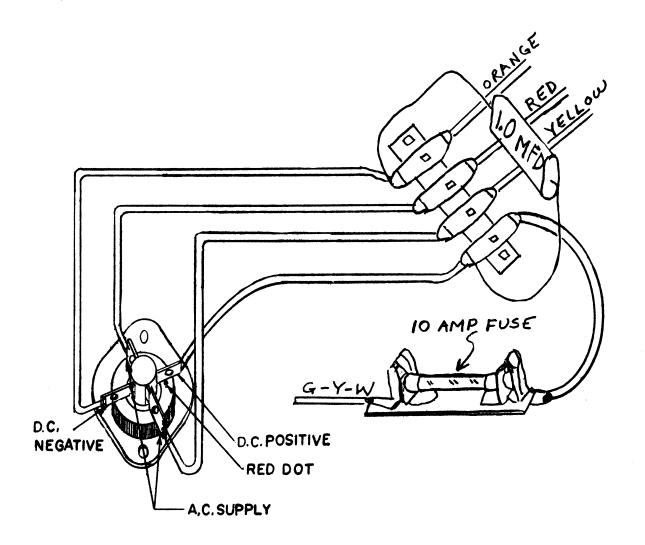
THE FUNCTION OF THE RECTIFIER AND CAPACITOR IS TO CONVERT THE ALTERNATING CURRENT (A.C.) TO DIRECT CURRENT (D.C.), SUPPLYING D.C. TO THE BUMPERS, KICKERS ETC.
