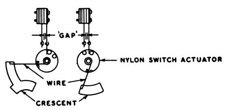
Long blade should be in contact with nylon switch actuator and have a maximum overtravel of 1/32.
