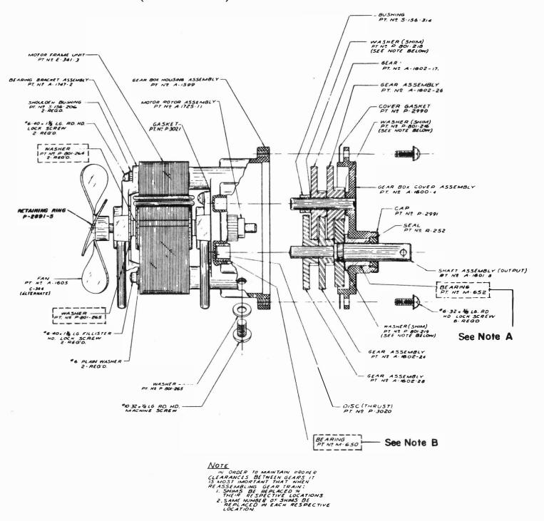
NOTE A: Bearing M-652 is part of Gear Box Cover Assembly A-1600-4 and cannot be ordered separately.
