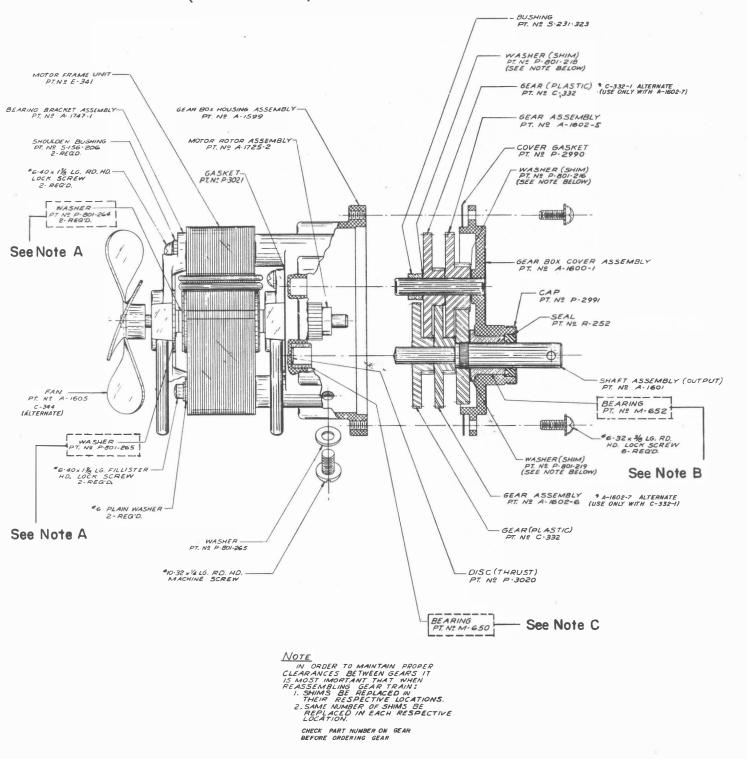
NOTE A; Washers P-80I-264 and P-80I-265 are parts of Motor Rotor Assembly A-1725-2 and cannot be ordered separately.
