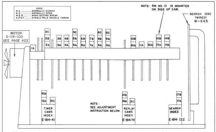
NOTE: IT IS IMPORTANT TO ADJUST REPLAY CAMS INDEX SWITCH NOS. 16A & 16B SO THAT THEY MAKE ONLY WHEN THE REPLAY CAMS INDEX COIL IS ENERGIZED. WHEN THE REPLAY CAMS INDEX IS DE-ENERGIZED, THESE SWITCHES SHOULD OPEN AND REMAIN OPEN WHILE SWITCH IS RIDING ON OUTER EDGE OF CAM.
