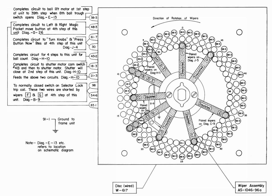
SCORE UNIT STEP-UP AND RESET AND RED AND YELLOW 3-IN-LINE SCORES 4-IN-LINE CIRCUIT
