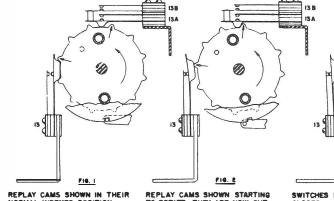
REPLAY CAMS SHOWN IN THEIR NORMAL INDEXED POSITION. SWITCHES ISA, ISB, & IS ARE OPEN AT THIS TIME. NOTE: ARROWS POINT TO LOBES THAT WILL ACTUATE SWITCHES.
