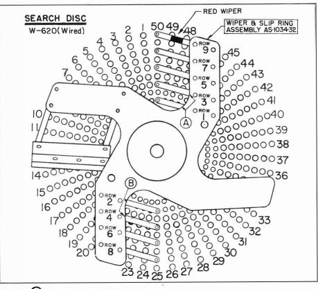
WIPERS (A) FED BY WIRE 80 (ON DIAG. C-15) THRU FEED WIPER. COMPLETES CIRCUIT TO SEARCH INDEX COIL AND REPLAY COUNTER STEP-UP COIL, WHEN SCORING REPLAYS. WIPERS (B) (ON DIAG. F-14) COMPLETES CIRCUIT TO SCORE 4 IN LINE SCORES – FOR 3 IN LINE, WHEN "RED" OR "YELLOW" RELAYS ARE TRIPPED.
