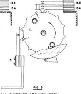
ALL SWITCHES ARE NOW OPEN AGAIN, SAME AS IN FIG. I. THIS SEQUENCE IS REPEATED THRUOUT REPLAY SCORING CYCLE.
