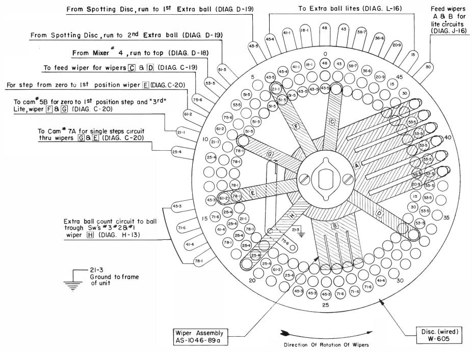
SHIFT UNIT (1st ROW) viewed from COIL side All 4 Shift Units are exactly alike from coil side All Coils and Switches shown approximate position on Diagram B-24
