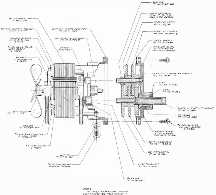
NOTE IN ORDER TO MAINTAIN PROPER CLEARANCES BETWEEN GEARS IT IS MOST INMORTANT THAT WHEN REASSEMBLING GEAR TRAINS I. SHIMS BE REPLACED IN THEIR RESPECTIVE LOCATIONS. 2. SAME NUMBER OF SHIMS BE REPLACED IN EACH RESPECTIVE LECENTION.
